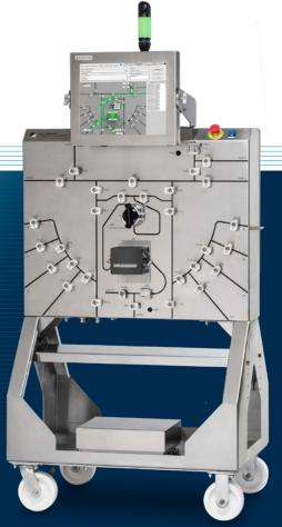
System design includes pinch valves for routing of fluid; pumps for flow and direction; flow, pressure and temperature transducers for process monitoring; and an in-line refractometer for fluid fractionation and monitoring.
